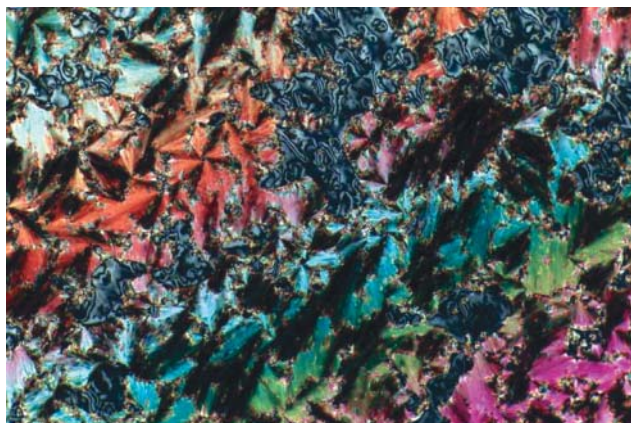
Fig. 1 S_C phase of compound 39 at 127.1 °C clearly showing broken focal conic domains accompanied by regions of pseudohomeotropic schlieren texture (100 × magnification).
